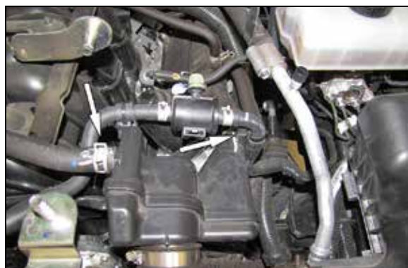
4. Release the spring clamps and then disconnect the crank case vent lines from the factory intake tube. Unhook EVAP hose retaining clips from the factory intake tube.
