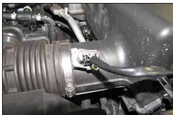
3. Disconnect the mass air sensor electrical connection and unhook the wiring harness from the air filter housing.
