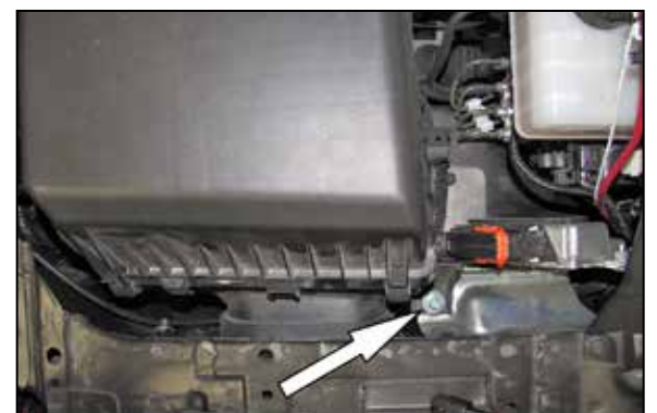
6. Remove the bolt shown that secures air filter housing to the inner fender and then lift the air filter housing up to dislodge it from the mounting grommets and remove it from the vehicle. NOTE: K&N Engineering, Inc., recommends that customers do not discard factory air intake.
