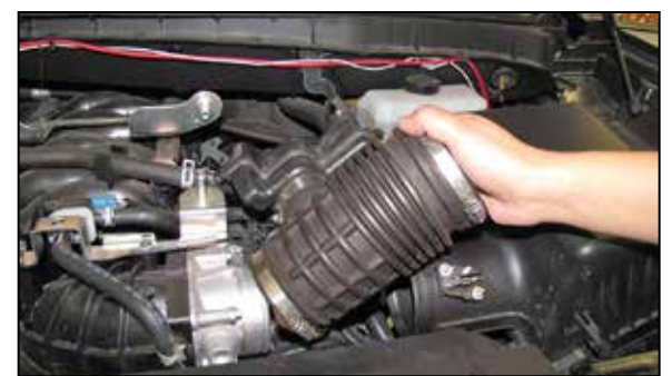
5. Loosen the two hose clamps that secure the factory intake tube and then remove the tube from the vehicle.
